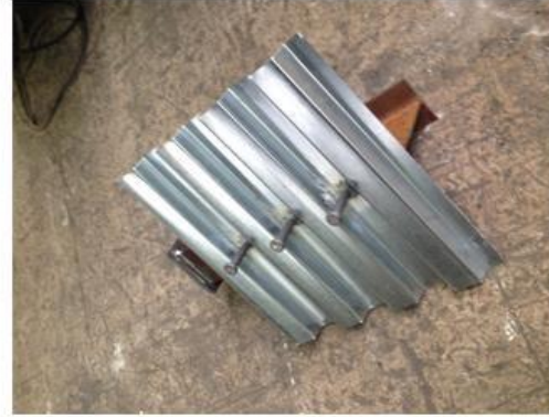
Figure2. Welded headed studs
