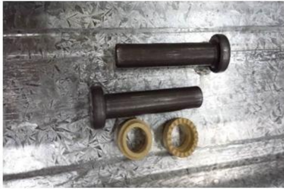
Figure1. Headed stud shear connectors
